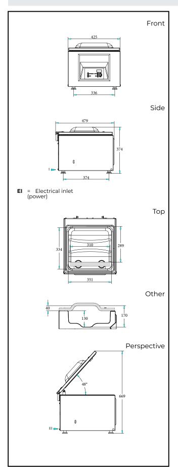
Supply voltage: 220-240 V/1N ph/50-60 Hz **Total Watts:** 0.6 kW Key Information: Filling board nr: 2 Gas nozzles: no gas External dimensions, Width: 425 mm External dimensions, 479 mm Depth: External dimensions, 374 mm Height: Net weight (kg): 35.5 **Well Capacity:** 14.1 lt Pump:  $8 \text{ m}^3/\text{h}$ Sealing bar position: Front Sealing bar length: 310 mm Max chamber (chamber + 334 x 351 x 170 mm cover) dimensions: Chamber working dimensions: 289 x 347 x 130 mm
